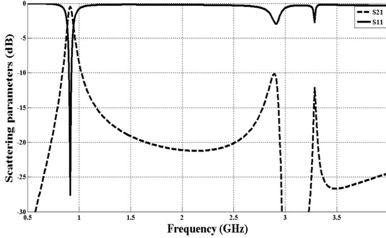
**Figure (5):** Layout simulation after adding the stepped impedance lowpass filter.
