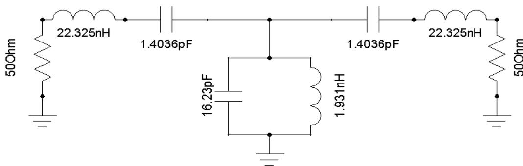
**Figure (1):** Circuit elements of the 900MHz bandpass filter.
