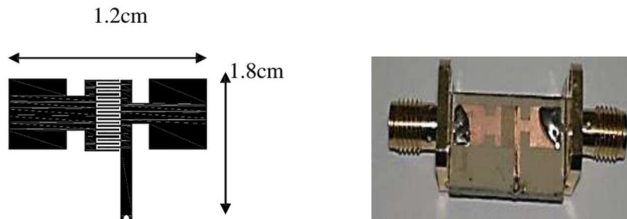
**Figure (6):** (a) Layout mask (b) Photograph of the fabricated UWB filter.
