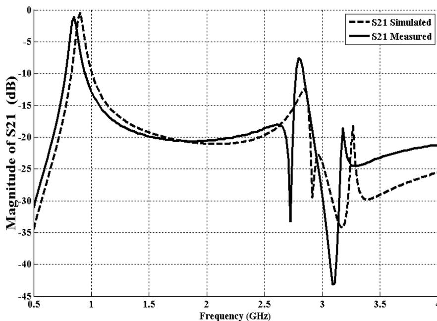
**Figure (7):** Insertion loss comparison of the measured and simulated results for the (900MHz) filter.
