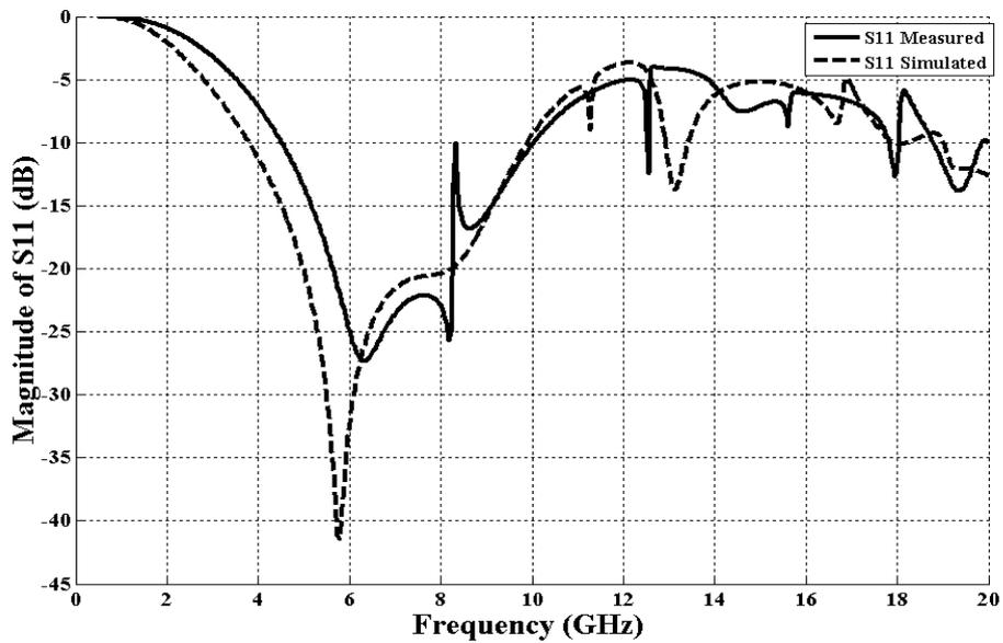
**Figure (10):** Return loss comparison of the measured and simulated results for the UWB filter.
