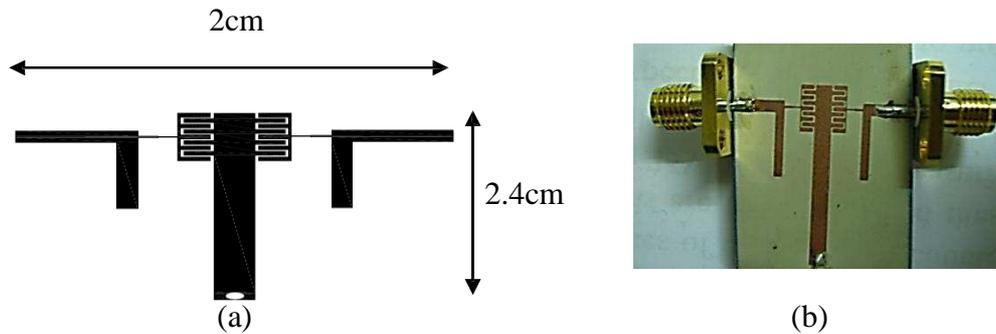
**Figure (4):** (a) Layout mask (b) Photograph of the fabricated 900MHz filter.
