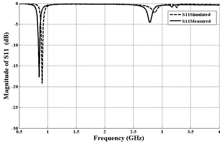
**Figure (8):** Return loss comparison of the measured and simulated results for the (900MHz) filter.
