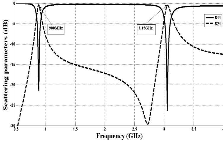
**Figure (3):** Layout simulation of the 900MHz bandpass filter.
