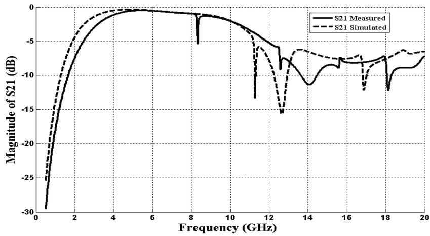
**Figure (9):** Insertion loss comparison of the measured and simulated results for the UWB filter.
