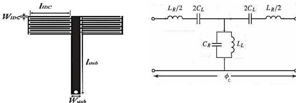
**Figure (2):** Unit cell T-equivalent.
